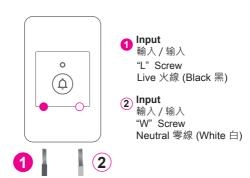
Screw the Wall Switch on the wall, than turn on the power at the switchboard. Installation completed.
